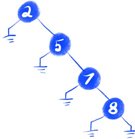
but it is no better than a linear list. The search for 9 in this tree is forced to visit every single node because it is *unbalanced*: some paths are very short (like the left-most path from 2, which immediately stops after one step) whereas some paths are very long (like the right-most path from 2 to 8, which has four steps).
